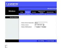
Wireless SSID Broadcast. When wireless clients survey the local area for wireless networks to associate with, they will detect the SSID broadcast by the Router. To broadcast the Router's SSID, keep the default setting, Enable. If you do not
